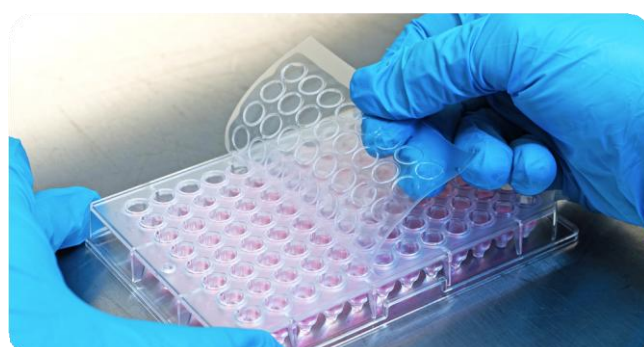
Figure 2: Hold the plate firmly with your left hand while applying downward pressure, then remove seal with your right hand until the whole membrane is released.
